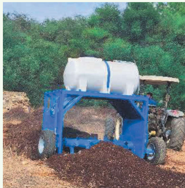
The ARI unit was equipped with a compost turner made by a local agricultural machinery manufacturer, at a low cost.
