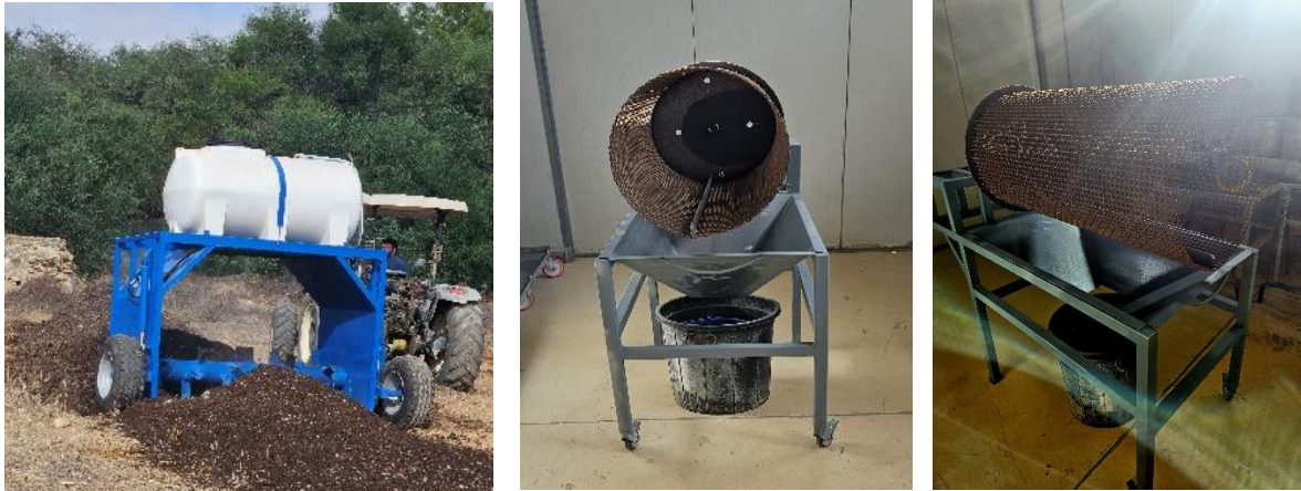
Figure 8: The compost turner and the sieving machine.
